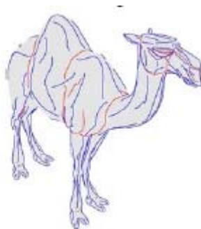
Fig. 2 Example of ridge lines used to convey the shape of a 3D surface
